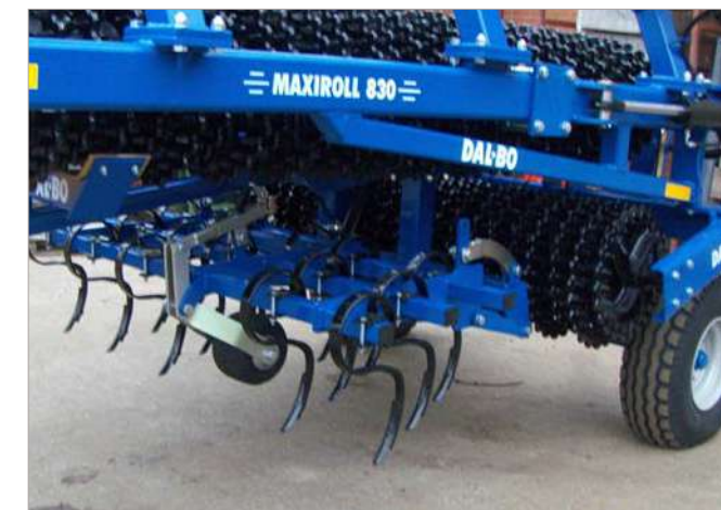
3 rows of heavy duty 45 x 10mm spring tines can be mounted to the front of the MaxiRoll.
