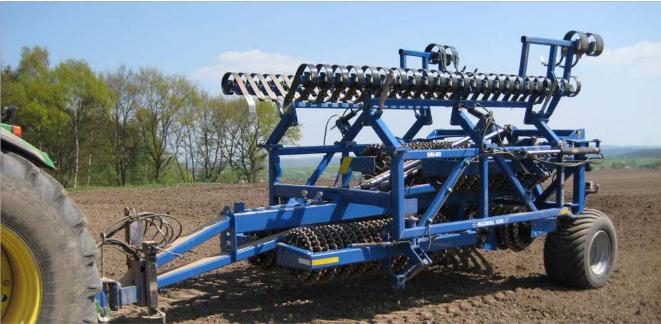
Crackerboard As standard the crackerboard is equipped with heavy duty 100 x 12 mm curved blades.
