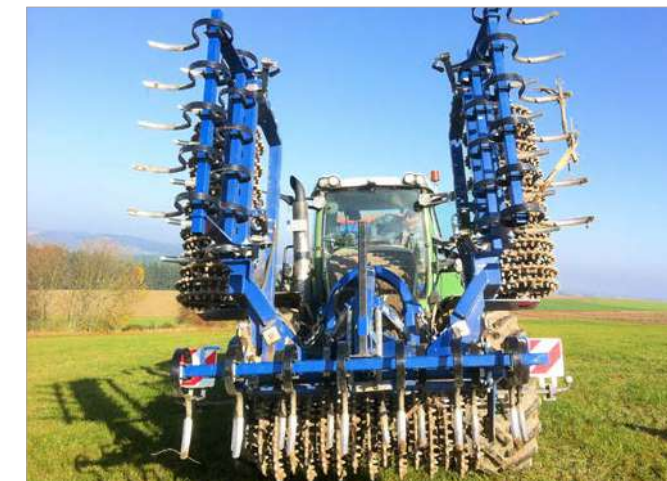
On the hydraulic folding 4m and 6m Levelflex models the hydraulic folding wing sections fold neatly to give a transport width of only 2.9m. The hydraulic folding models are fitted with an automatic mechanical locking device for transport.
