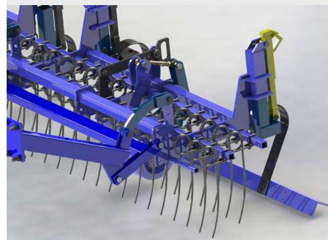
2 rows of tines with mole hill board
