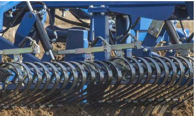
Secure fixation with bolts to a flange welded to the main frame. Spindle adjustment of cracker board is held in a parallelogram ensuring same working angle irrespective of the working depth
