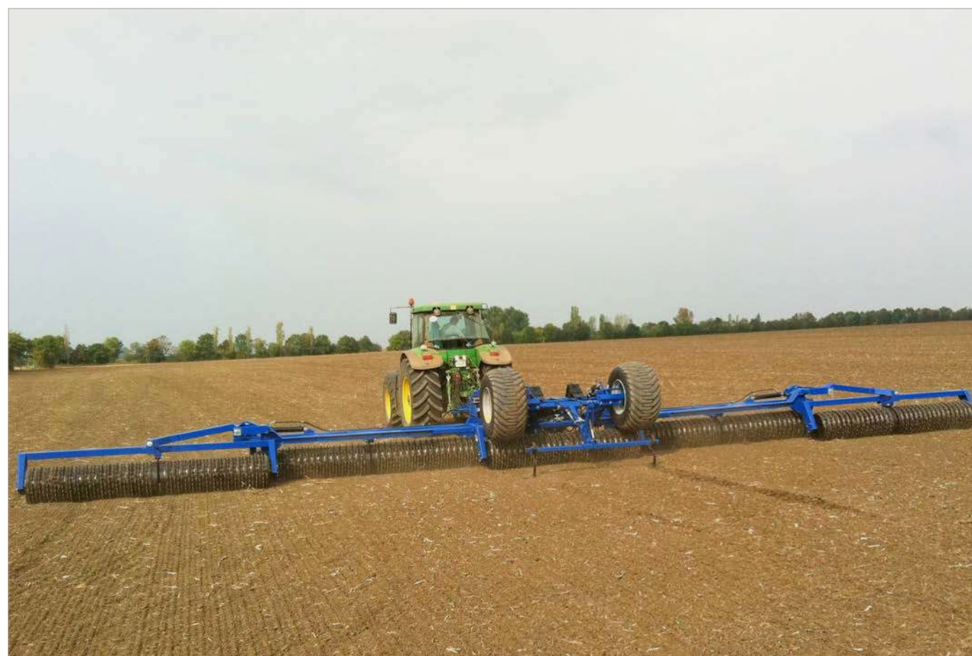
16.3m PowerRolls fitted with pre-emergence markers
