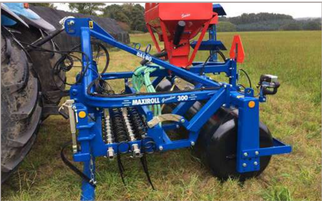
Greenline 300 with 710mm steel drum
