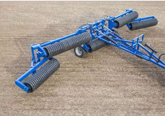
..... once the wings sections have been fully unfolded they are ready to be lowered into the working position
