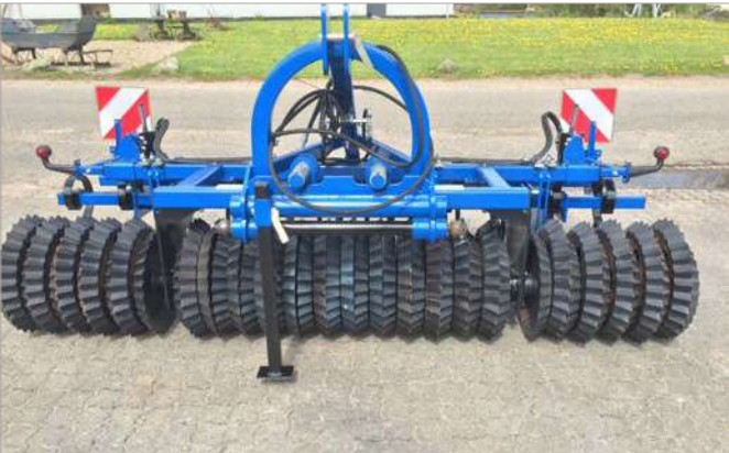
FrontFlex fitted with cross combi rings, lights and parking stand.
