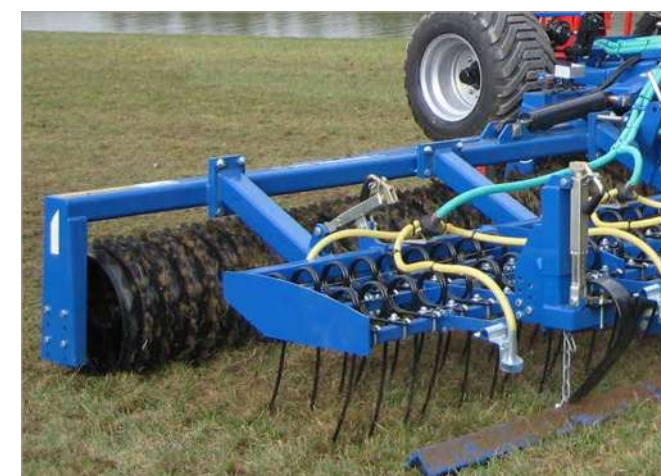
2 rows of 12mm harrow tines in combination with a mole hill board
