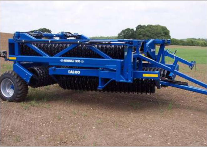
First the wing sections are lifted out of the transport locks.....
