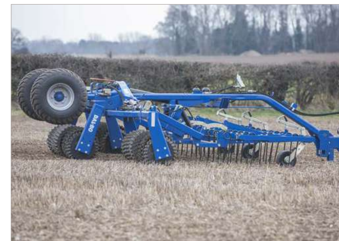
6.3m Maxiroll fitted with a BlackGrass harrow of 4 rows of 16mm heavy duty straight tines.
