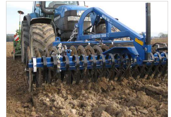
The front mounting and improved geometry actually means that the implement is being 'pulled' forwards, making it easier to steer.
