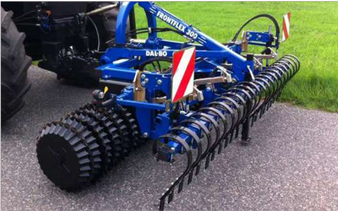
FrontFlex fitted with spindle adjusted cracker board
