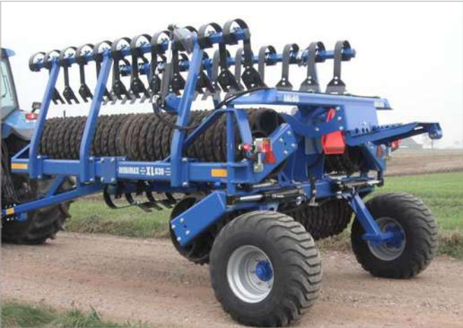
MiniMax XL with hydraulically adjustable cracker board
