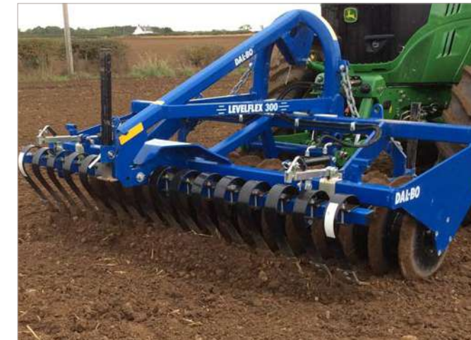
3m LevelFlex shown with hydraulic cracker board and the Dal-Bo 'V' profile packer
