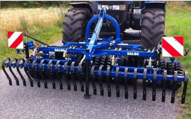
Spindle adjusted crackerboard
