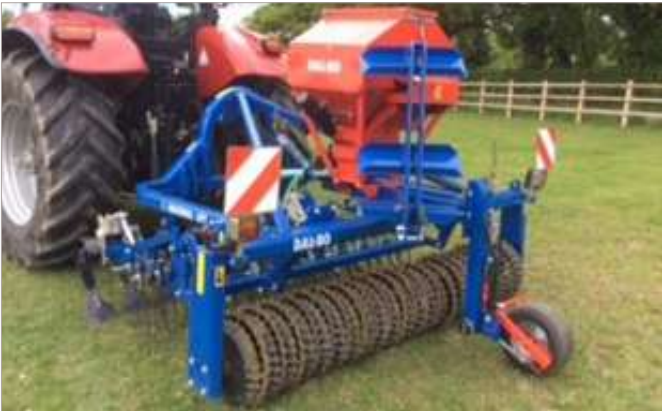
Greenline 300 with 3-point linkage is a modern solution to grassland management and a good implement for maintaining of existing grassland, sports centres, golf courses, hors pens etc.
